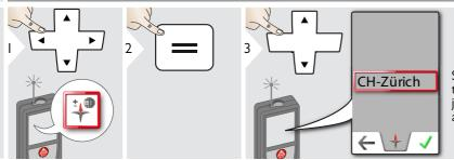
Select the nearest location and the device adjusts the declination accordingly.
