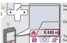
Switch between measurements.
