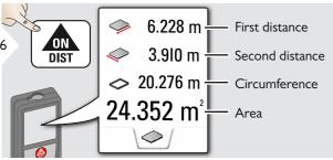
The result is shown in the main line and the measured value above. ment. Measure and add or subtract distanc-
