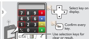
The measurement result from the main line is taken over to the calculator and can be used for further calculations.
