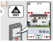
Select arrows with the cursor keys or by tapping on the display and adjust with softkeys. Corresponding width is calculated.
