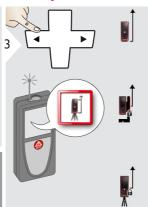
Distance is measured from the rear of the device (standard setting).
