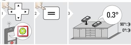
Displays inclinations of 360° with a strument beeps at 0° and 90°. Ideal for horizontal or vertical adjustments.
